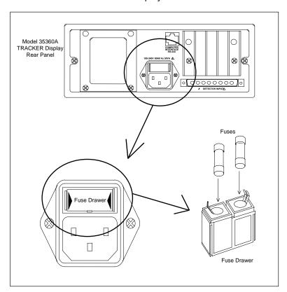
Figure 4-6. Model 35360A TRACKER Display Fuse Replacement
